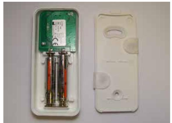
Suggested placement of supplied sticky pads are shown in the photos above. The tabs can be tucked inside the case before fastening the back into place. This will stop the tabs from protruding out of the sides once fitted into position.
