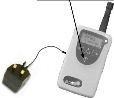
Charger can be left permanently connected or it can boost charge from empty in 8 hours
