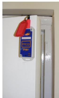
The unit is housed in small 40\*110mm case, powered by a Lithium Coin Cell for up to 1 year, with an alarm on battery low. It is compatible with the P137 pager which can monitor up to 32 such alarms (or the P138 for 3 users) or the P117C Telephone Autodialler
