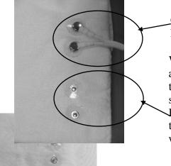
Connect sensing lead lead to here (P141)
