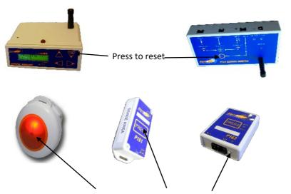
Press for 1 second until LED stops flashing (and beep heard on some units)
