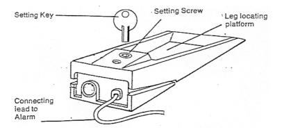
The unit must be calibrated for the bed weight to ensure maximum sensitivity to the user. This requires the use of an indicator to show operation of the unit, and inherent feature with the P154 pr P139 Bedside Monitors.
