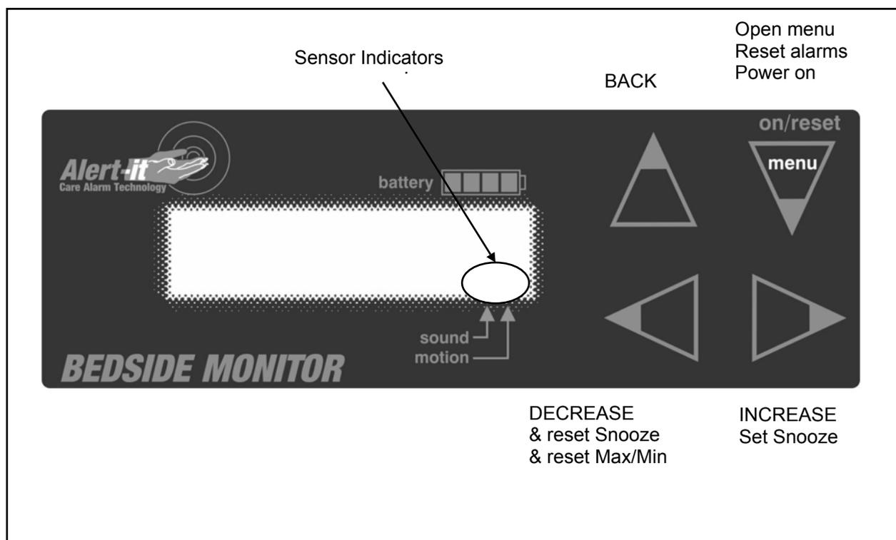
A liquid crystal display screen with back lighting and a touch sensitive keypad is provided in order to indicate and adjust, as required, the functions and the status of the system.
